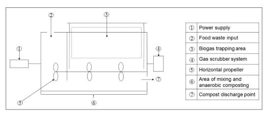
Figure 1. Schematic diagram of pilot-scale anaerobic composter
