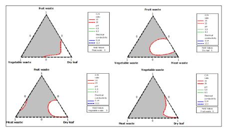
*Figure 3.* Overlaid contour plots of C/N ratio, pH and electrical conductivity of food wastes with dry leaves composting
